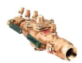
Reduced Pressure Zone Backflow Preventer: WATTS LF009, 2 in, IPS, Lead Free Bronze, 21 3/8 in Lg
